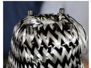
(Fig 2: example of loose tie off of braid to facilitate full fabric saturation)
