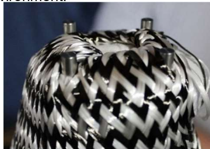
(Fig 2: example of loose tie off of braid to facilitate full fabric saturation)
